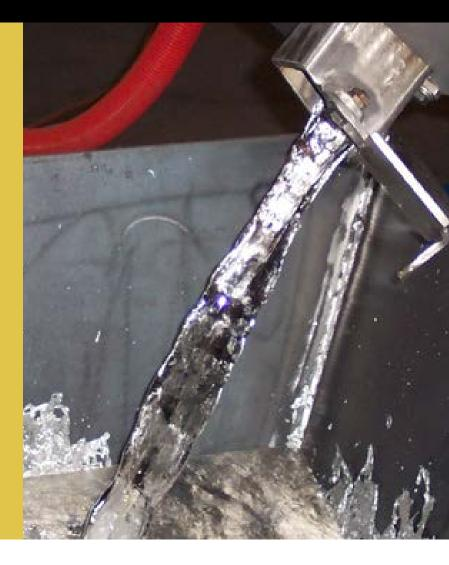
Zinc metal is entrapped in the floating ash created by the galvanizing process. The ash is skimmed from the galvanizing bath and loaded directly into the specially fabricated barrels. The barrels are then transferred to the reclaimer for processing.
