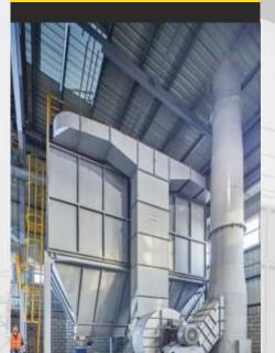
The fumes collected in the fume enclosure are filtered in the bag filter.
